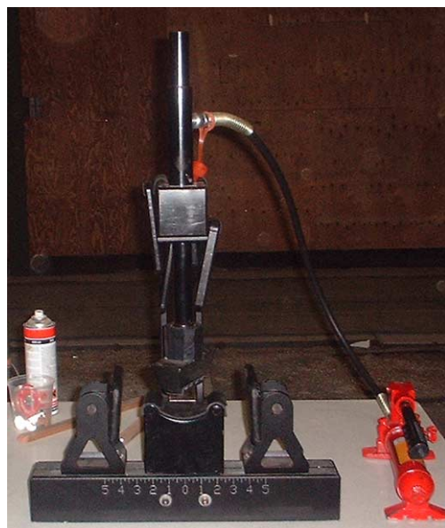
Fig. 1. The tree machine used to adjust tree size and angle by putting pressure on the inner side of the tree.
